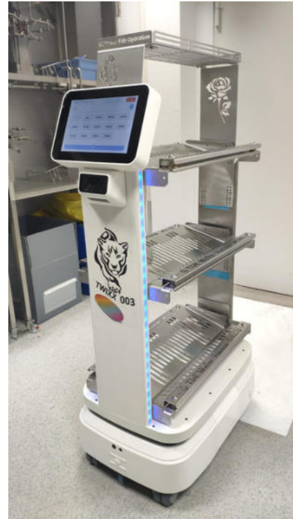
Transport-Roboter Autoxing 6113 - 150 kg
